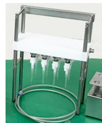
① AHST-16HB Heat block for 16 vials ② AHST-16TC Temperature controller for 16 vials
