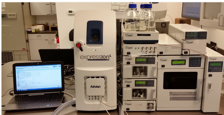
Figure 1: UHPLC-CMS set up for the detection and quantification of amino acids in complex mixtures utilizing a JASCO X-LC system (Jasco, USA), an Intrada Amino Acid HPLC column (Imtakt Corporation, Japan) and the expression L compact mass spectrometer (Advion, Inc. USA).
