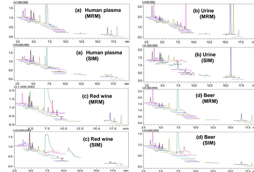
Figure 4: MRM (top) and SIM (bottom) profiles of (a) human plasma, (b) urine, (c) red wine and (d) beer sample.
