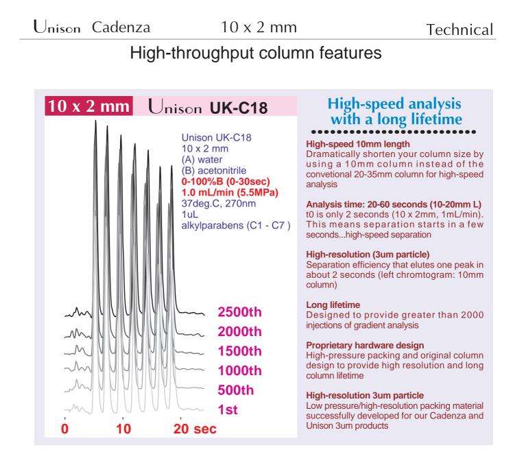
Conventional high-speed analytical columns are 20-35mm in length. Some manufacturers provide 10mm length columns as a cheap cartridge but these suffer from poor column lifetime.
