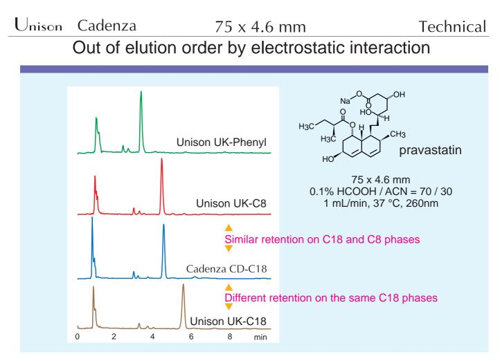
Unison series are compatible with 100% of aqueous eluent, and designed to provide better retention and separation for hydrophilic compounds. In contrast, Cadenza CD-C18 phase is designed with high ODS density to achieve better molecular recognition due to large steric selectivity.
