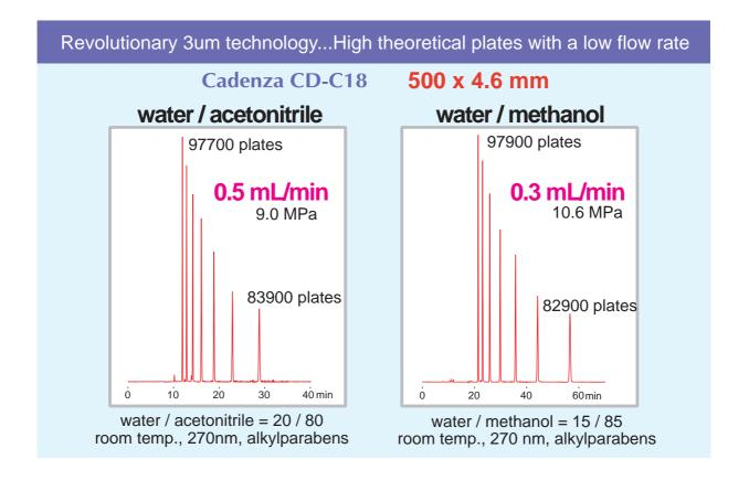
Cadenza CD-C18 500 x 4.6mm is a high-efficiency column offering 100,000 plates per column in resolution. Researchers typically use a flow rate of 1mL/min with a 4.6mm I.D. column. In many cases with a 3um particle, this results in high pressure and difficulties for researchers. For that reason, it is necessary to lower the flow rate when using our 500mm column.
