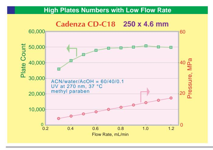
This chromatogram shows the relationship between plate numbers and flow rate for the high-resolution Cadenza CD-C18.
