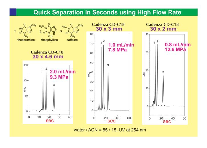
This data shows the impressive high-speed separation achieved by using the small column Cadenza CD-C18.
