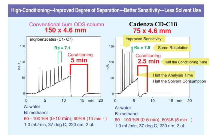
Cadenza CD-C18 has revolutionized the conventional standard size 150 x 4.6mm column.
