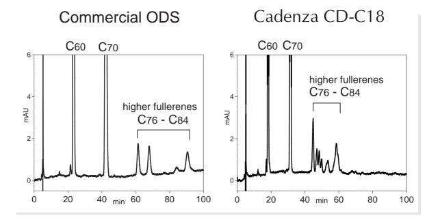
250 x 4.6 mm, hexane / 2-propanol = 40 / 60 0.6 mL/min, 30 °C, UV at 325 nm
