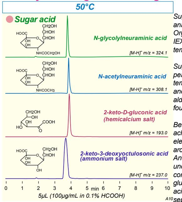
Sugar acids can also be analyzed on the Intrada Organic Acid column, using IEX mode and high temperatures.
