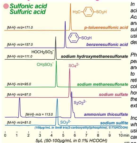
In addition to carboxylic acids, the Intrada Organic Acid column is also able to analyze stronger acids, like sulfuric or sulfonic acids using IEX mode and MS detection.
