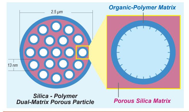
The advantage of using traditional silica-based particles is that they have a high mechanical strength; their disadvantage is that they are prone to degradation under alkali conditions. On the other hand, polymer-based particles are highly resistant to degradation under alkali conditions, but they suffer from poor performance and durability due to shrink/swelling effects when used with organic solvents.
