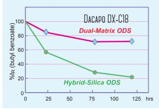
Even though hybrid-silica columns are resistant to alkali degradation, surface silanols are still susceptible to hydrolysis under high pH conditions. The surface silanols of DACAPO are completely covered with an organic polymer layer, dramatically improving alkali stability.
