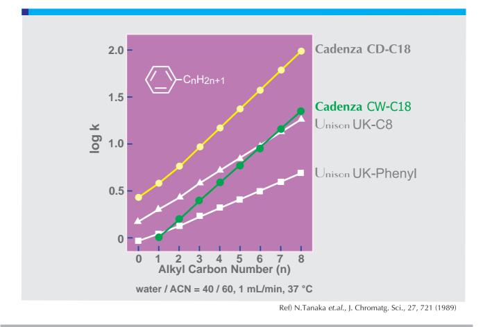
Cadenza CW-C18 is a high-throughput and high-resolution ODS phase which consists of 3um silica particle and 30nm pore size. The specific surface area of CW-C18 is 1/3 of Cadenza CD-C18 due to the larger pore size - resulting in less retention than a conventional ODS phase.
